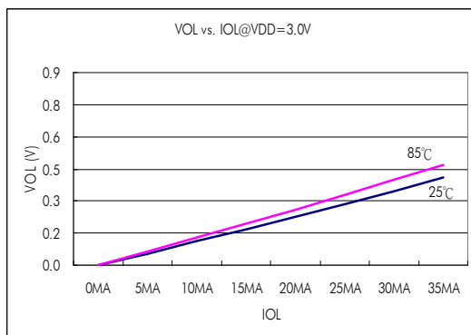
Figure 6.4-3 V_{OL} vs. I_{OL} @ V_{DD}=3.0\text{V}
